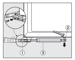
■ Leave the hinges open and remove the screw in the mounting ①.
